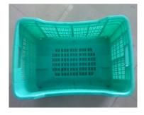
Feedback to plant: Eliminate warpage in side walls.
