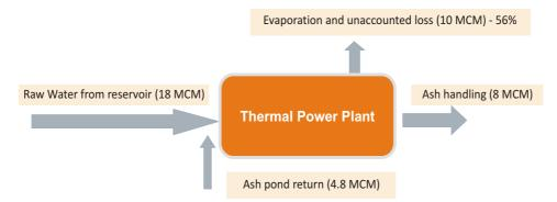
Figure 2: Water balance of a coal based power plant
