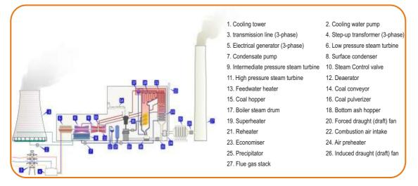
Figure 1: Schematic diagram of thermal power plant<sup>1</sup>
