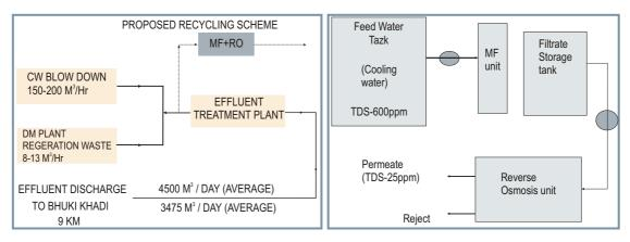
The water quality of the RO outlet was compared with the raw water and was found to be better than the raw water. A comparison of the CT blown down water, raw water with the RO outlet water indicates the suitability of the RO water for use in the DM plant as compared to raw water.
