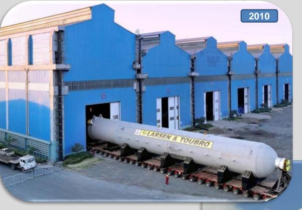
KNPC Hydrocracker Reactor – 1540 MT, 308mm
