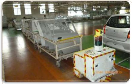
Automatic Guided Vehicles (AGV) for Door transfer "Zero Handling Dents"
