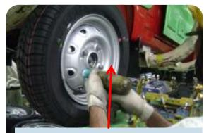
Auto-Torque regulator to prevent over tightening
