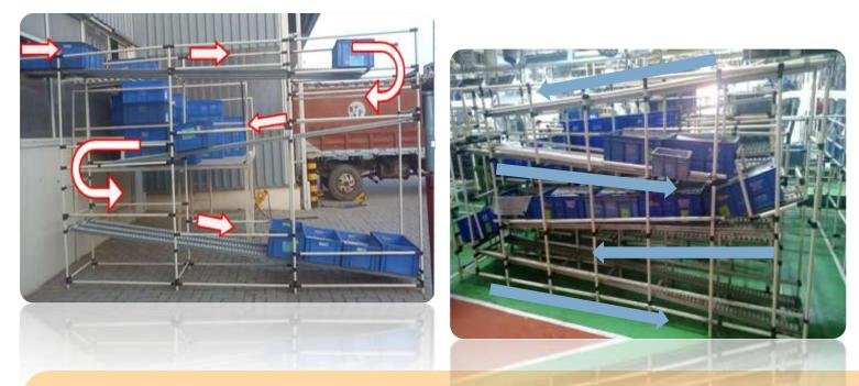
Tak-a-Tak systems for continuous transfer of material, utilising vertical space, with 'o' manual intervention
