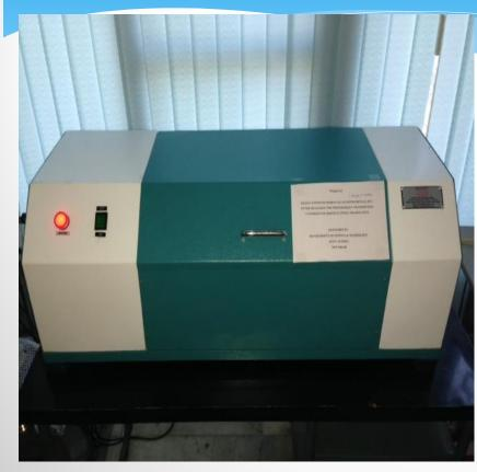
Light Source : Tungsten filament with 400 -700 nm wavelength
