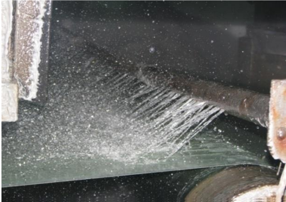
Fig 3: Inefficient Hole Showers consuming more water
