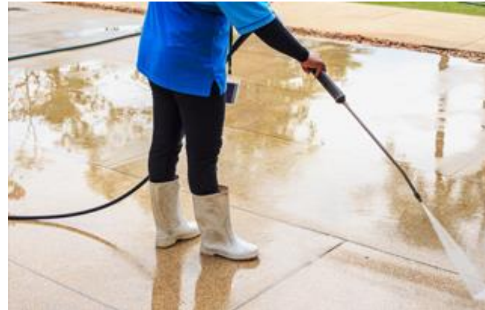
Suggested - Curtain type spray nozzle with pressurize water hand control lever for effective floor cleaning
