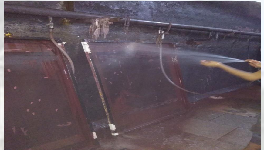
MIX WATER (R.O. REJECT+ETP) FOR SCREEN WASHING at VIRAJ
