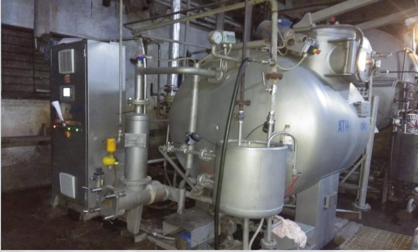
FULLY AUTOMATED (PLC) SOFT FLOW DYEING M/C at GINZA INDUSTRY
