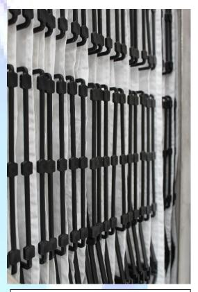
The ceramic gills with air spacers provide the perfect oxygen/liquid interface for microorganisms to flourish.
