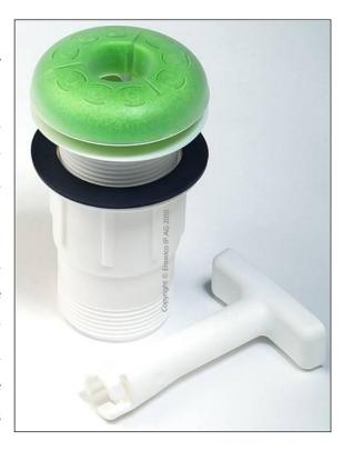
The Key-Valve automatically balances negative pressures in the drain line as the Key-Membrane allows air to flow into the drain. When the line is under pressure, the Key-Membrane remains tightly closed.
